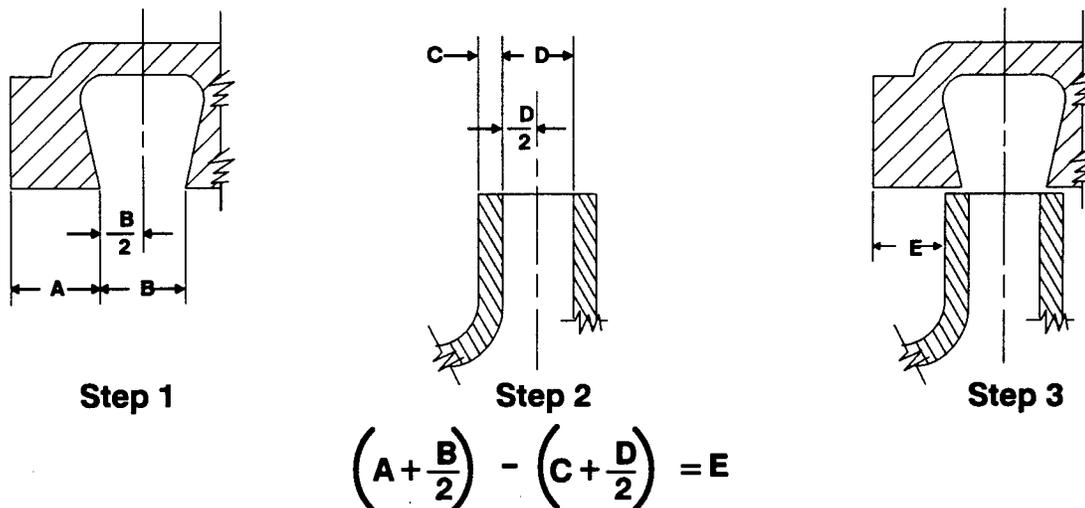
**Figure 4. Centering Impeller Within Pump Casing**
