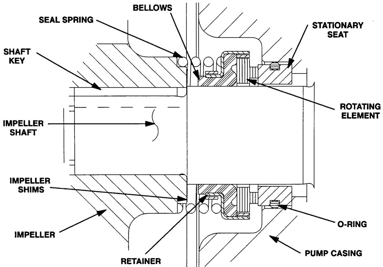
Figure 2. 25271-192 Seal Assembly
