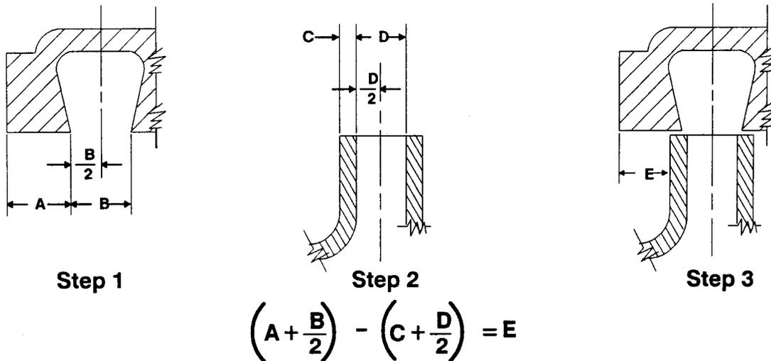
Figure 4. Centering Impeller Within Pump Casing
