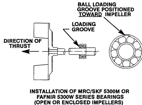
**Figure 5. Double Row Bearing Installation**
