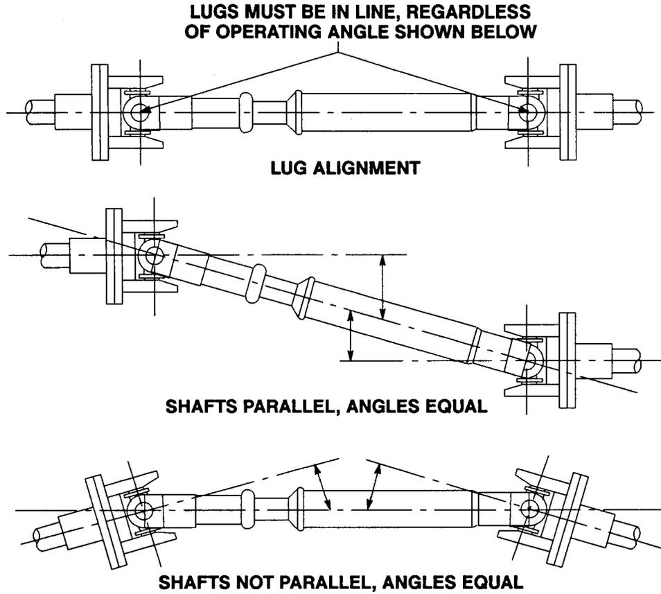
Figure 2. Proper Installation And Alignment of Universal Assembly
