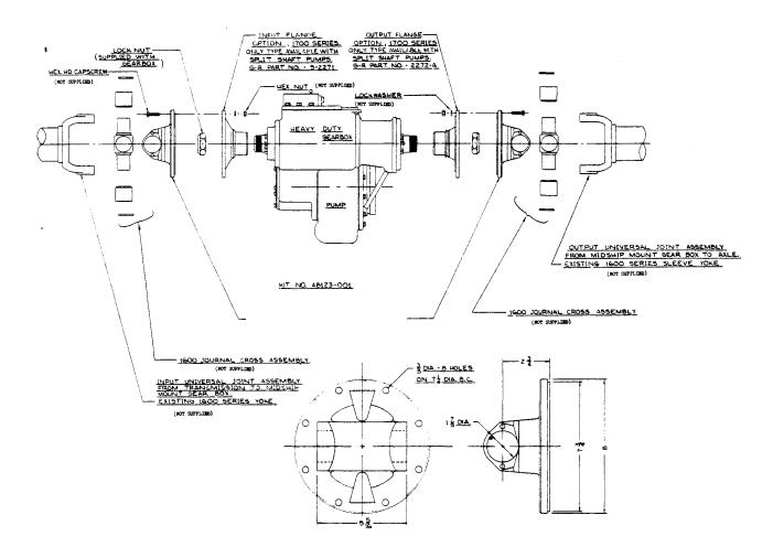
Figure 6. Adaptor Flange Yoke Installation
