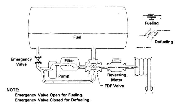
Figure 1. Typical Pumping Systems for Fueling Vehicles
