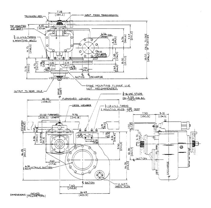
Figure 2. Dimensions of Pump Model 06C3-GH1
