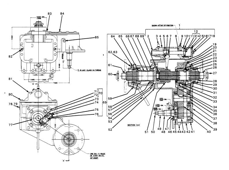
Figure 3. P/N 14017 Gear Box Assembly For Pump Model 06C3-GH1
