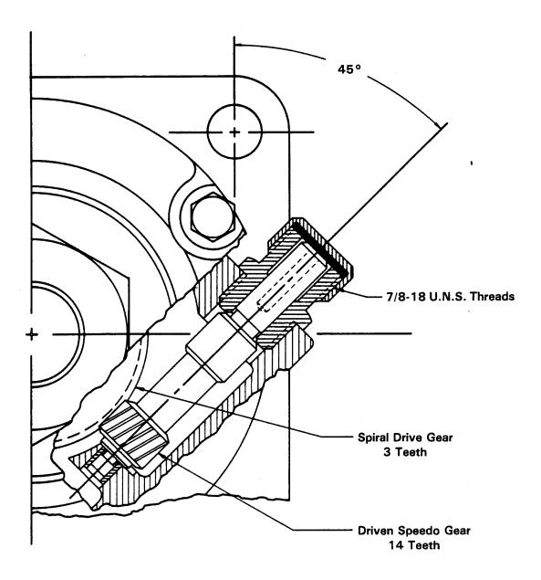
Figure 4. Speedometer Drive Detail
