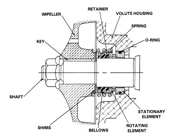
Figure 2. 25271-192 Seal Assembly
