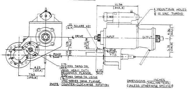
Figure 7. Typical 06 Pump Model With Stub Shaft PTO (Modified Version Available From Factory Only)
