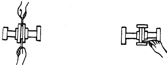
Figure 2B. Aligning Non-Spider Type Couplings
