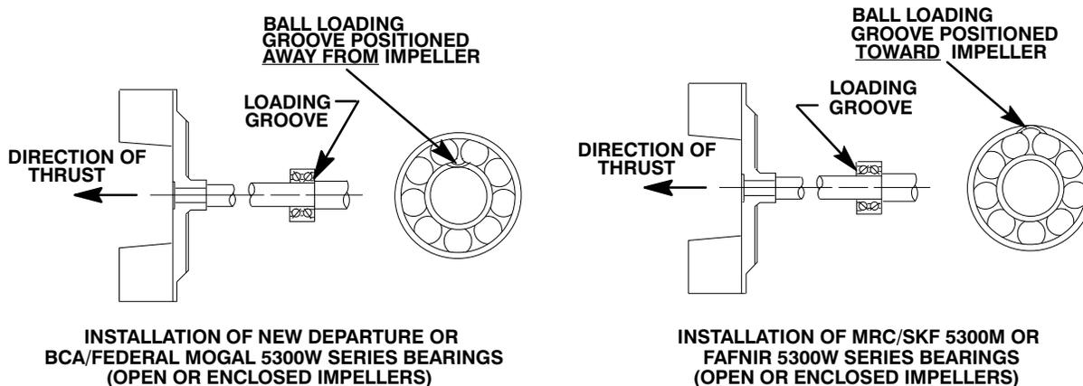
**Figure 2. Bearing Positioning**
