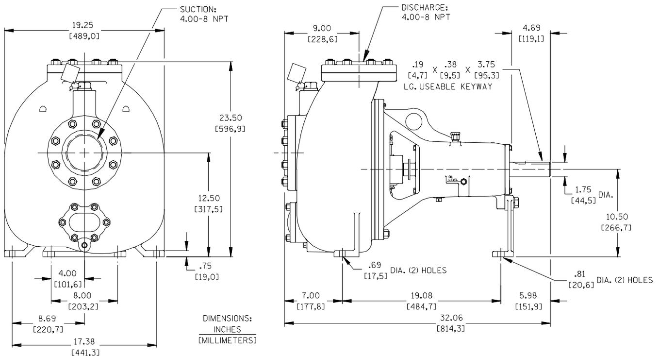
Figure 1. Pump Model 04B52-B
