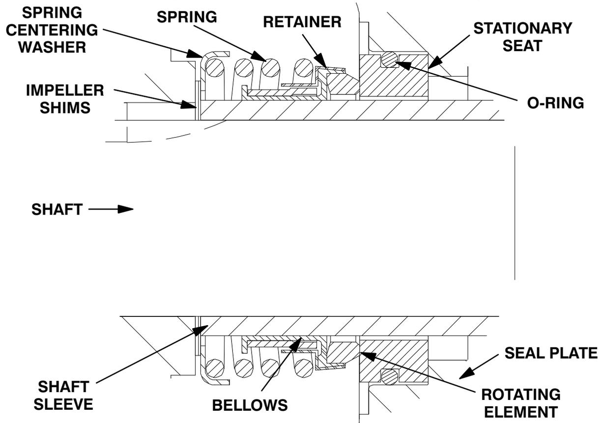
Figure 3. 25285-856 Seal Assembly
