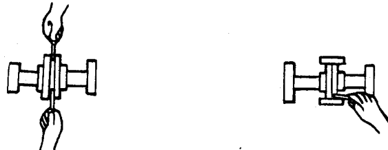
Figure 2B. Aligning Non-Spider Type Couplings
