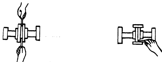
Figure 2B. Aligning Non-Spider Type Couplings
