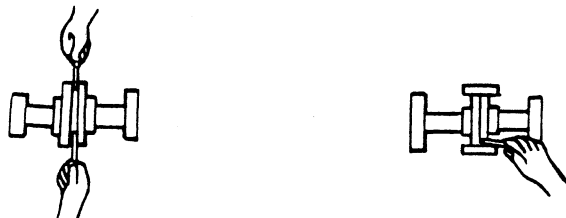
Figure 2B. Aligning Non-Spider Type Couplings
