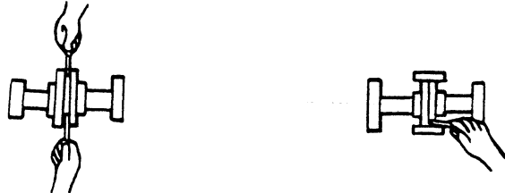
Figure 2B. Aligning Non-Spider Type Couplings
