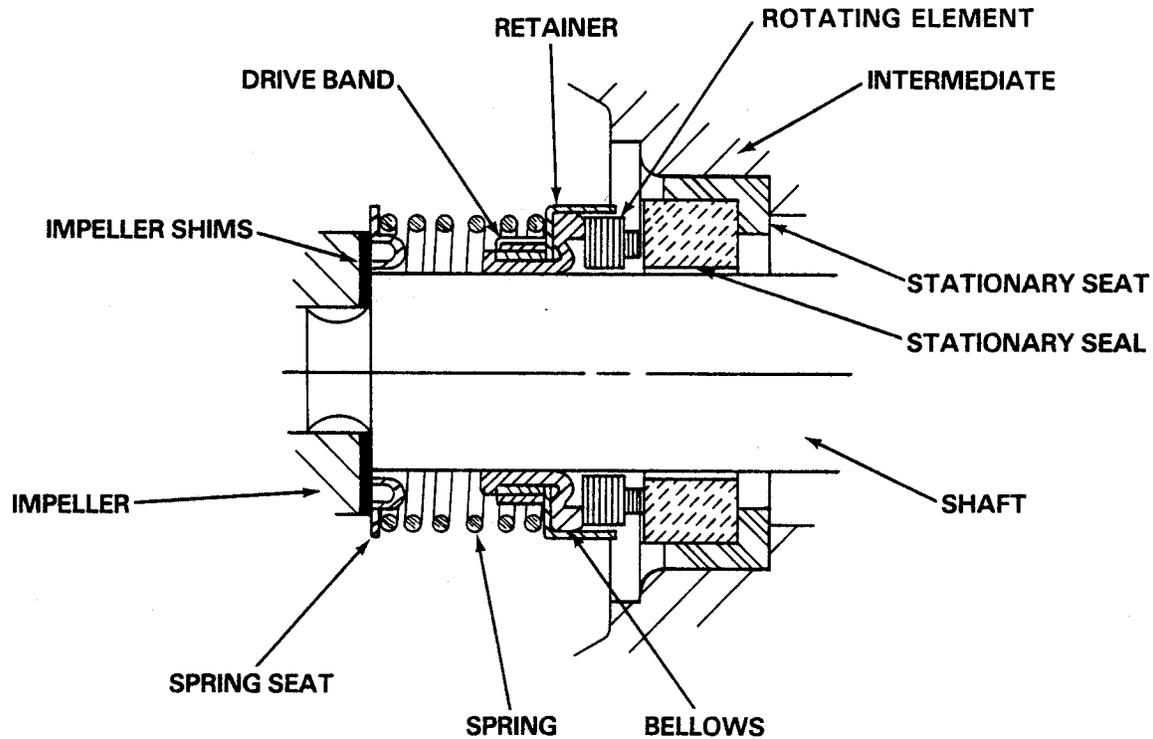
Figure 2. 25271-821 Seal Assembly
