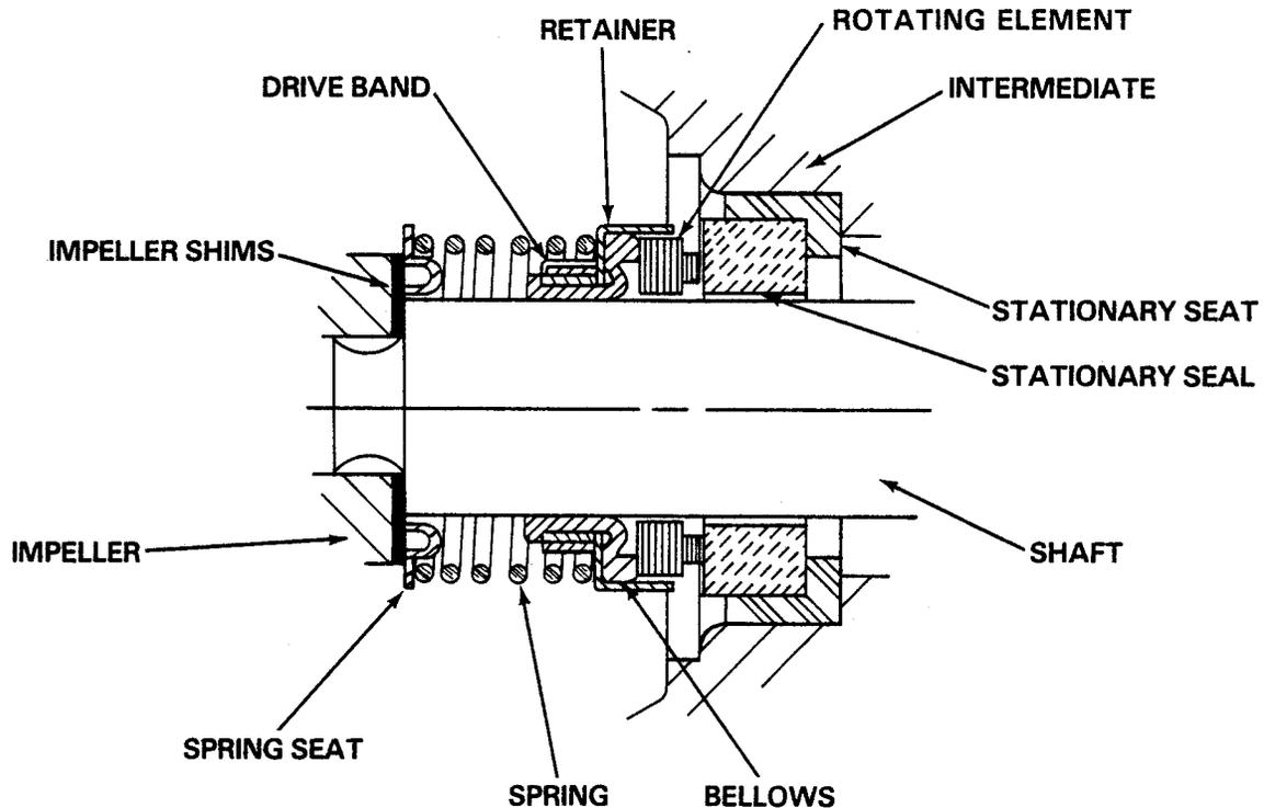
Figure 2. 25271-821 Seal Assembly
