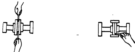
Figure 2B. Aligning Non-Spider Type Couplings
