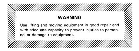
Make sure that hoists and other lifting equipment are of sufficient capacity to safely handle the pump assembly. If chains or cables must be used, make certain that they are positioned so that they will not damage the pump, and so that the load will be balanced.
