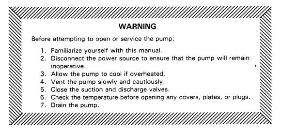
Disconnect the power source, making certain that it will remain inoperative while the pump is being serviced, and close all connecting valves.
