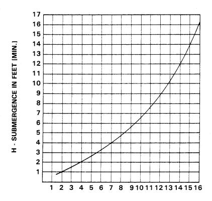
VELOCITY IN FEET PER SEC. =  $\frac{\text{QUAN. [G.P.M.]} \times .321}{\text{AREA}} \text{OR } \frac{\text{G.P.M.} \times .4085}{\text{D}^2}$
