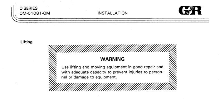
Make sure that hoists and other lifting equipment are of sufficient capacity to safely handle the pump assembly. If chains or cables must be used, make certain that they are positioned so that they will not damage the pump, and so that the load will be balanced.
