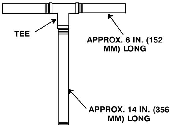
Figure 4. Rotating Assembly Tool
