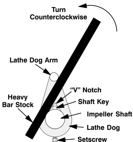
Figure 3. Loosening Impeller
