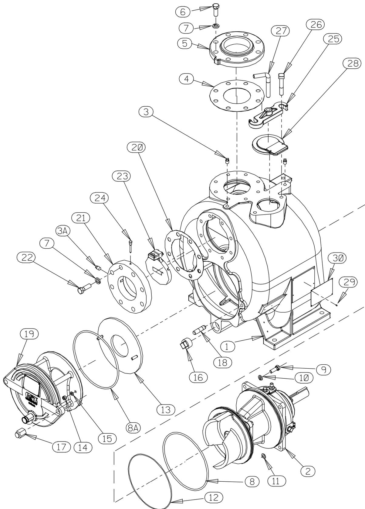
Figure 1. Pump Model T4A3-B, Including /F, /FM
