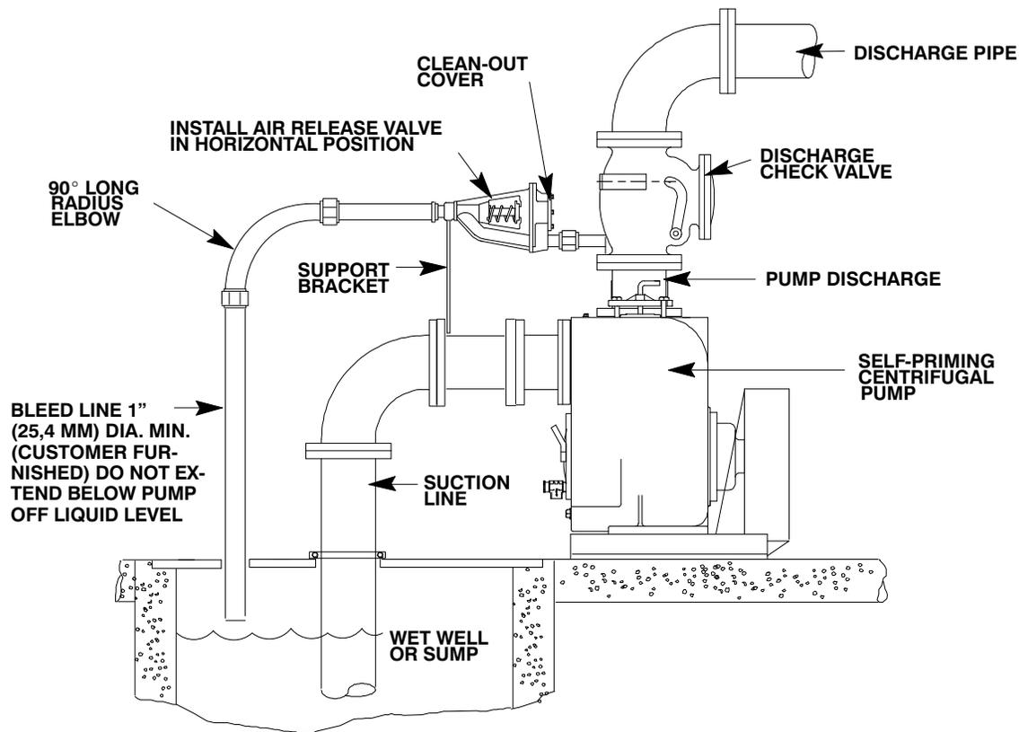
Figure 3. Typical Automatic Air Release Valve Installation
