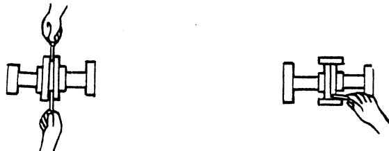
Figure 5A. Aligning Non-Spider Type Couplings
