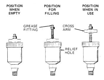
Figure 4. Automatic Lubricating Grease Cup
