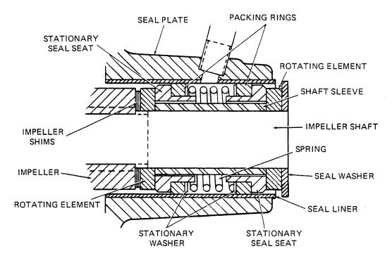
Figure 3. GS-1250 Seal Assembly
