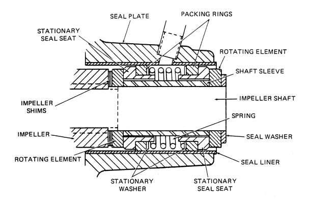
Figure 3. GS-1250 Seal Assembly
