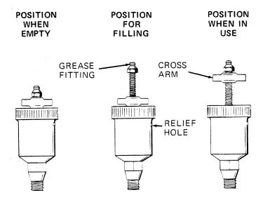
Figure 4. Automatic Lubricating Grease Cup
