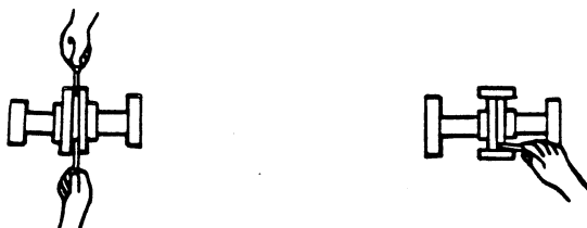
Figure 3B. Aligning Non-Spider Type Couplings
