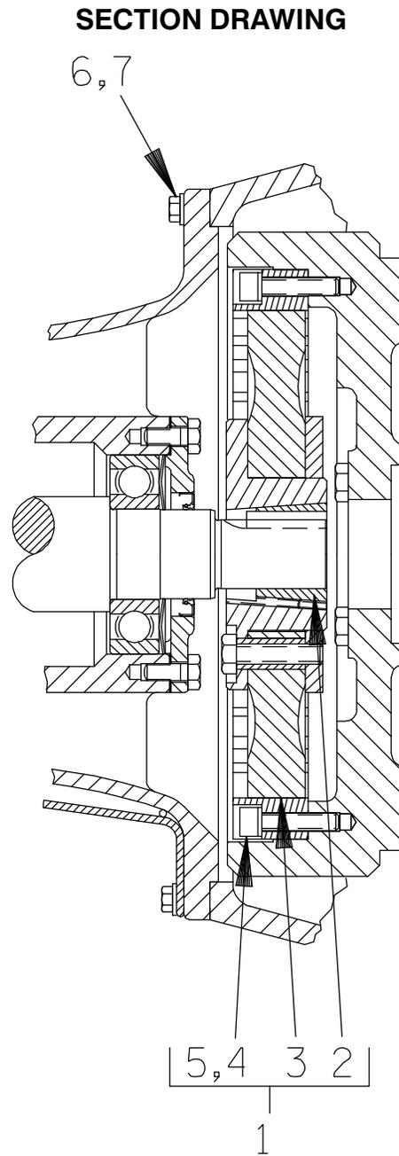
**Figure 3. Drive Assembly For Pump End 86A2-(SAE 4/10)**
