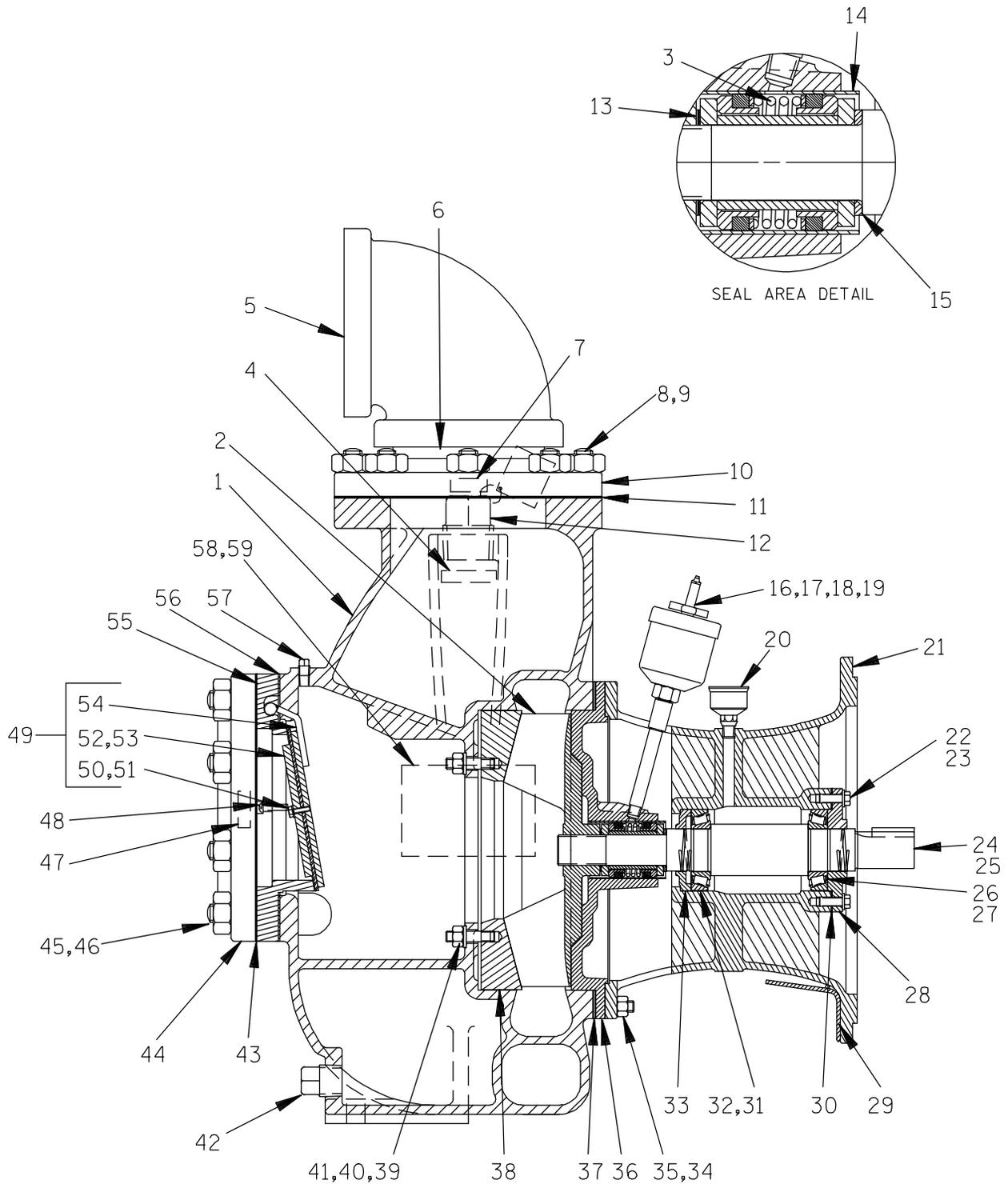
Figure 2. Pump End Assembly 86A2-(SAE 4/10)
