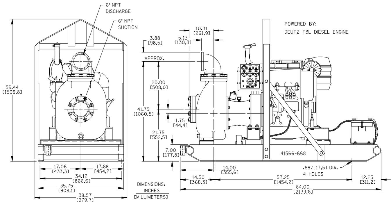
Figure 1. Pump Model 86A2-F3L
