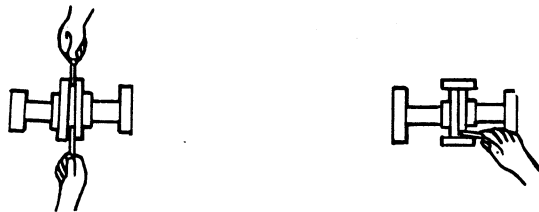
Figure 5A. Aligning Non-Spider Type Couplings
