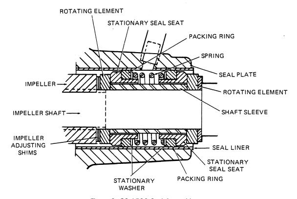
Figure 3. GS-1500 Seal Assembly
