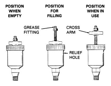
Figure 4. Automatic Lubricating Grease Cup
