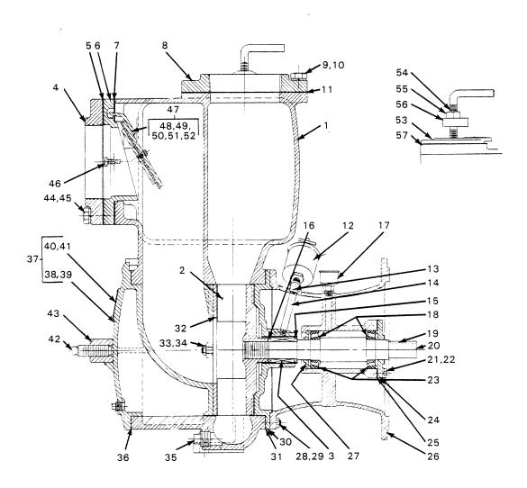
Figure 1. Pump Model 16A5-5034 Pump End Assembly
