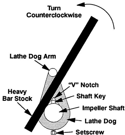
Figure 2. Loosening Impeller
