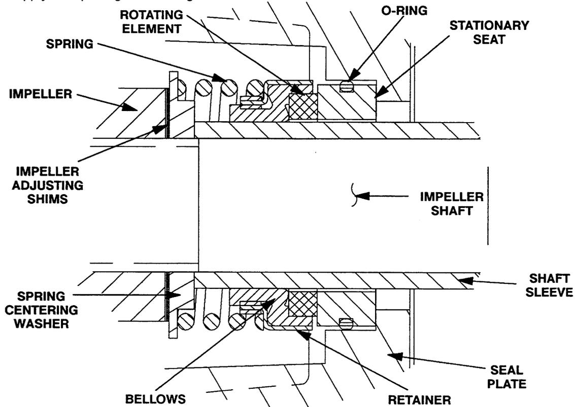
Figure 2. 25284-951 Seal Assembly
