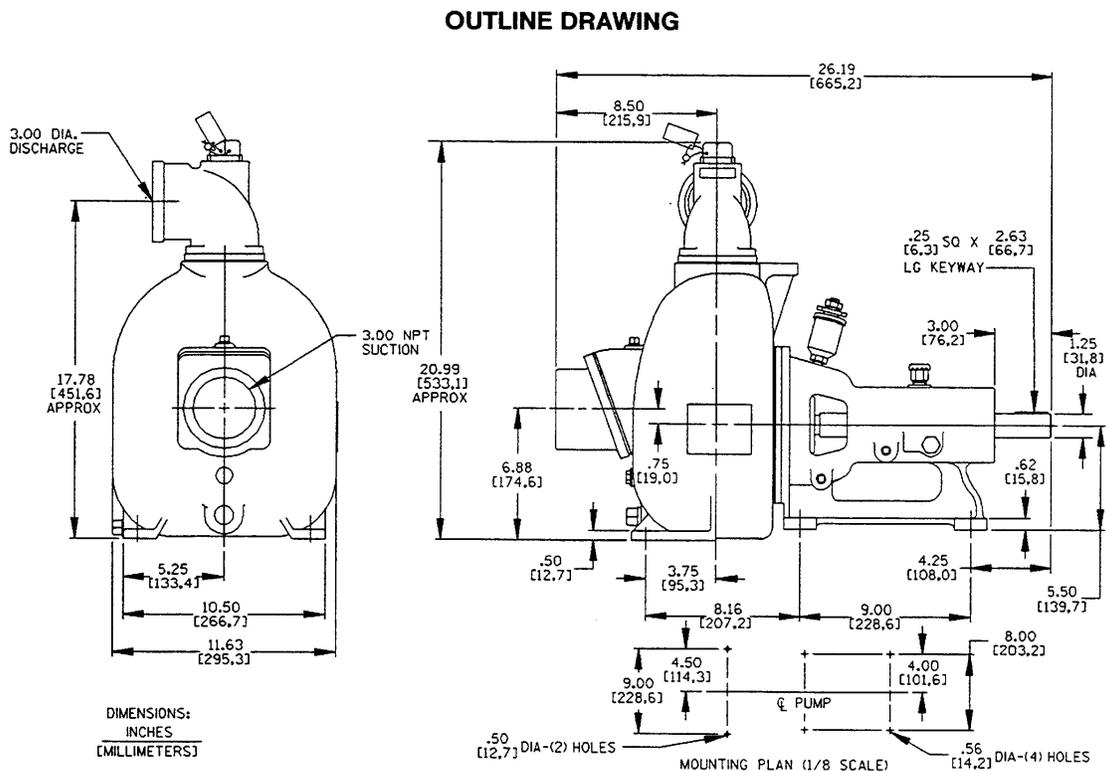
Figure 1. Pump Model 83B52-B
