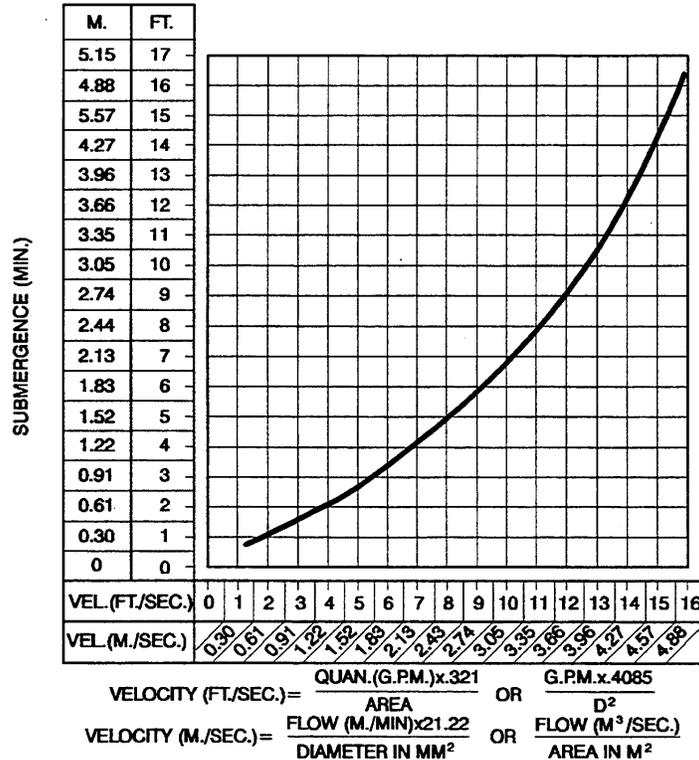
Figure 2. Recommended Minimum Suction Line Submergence vs. Velocity
