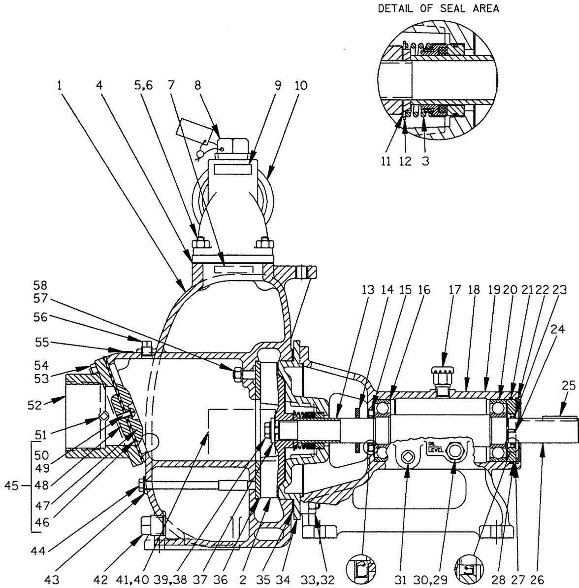
Figure 1. Pump Model 83B52-B
