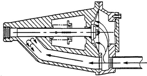
**Figure 2. Valve in Closed Position**
