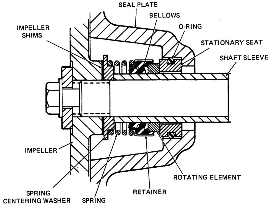
Figure 2. 25284-951 Seal Assembly
