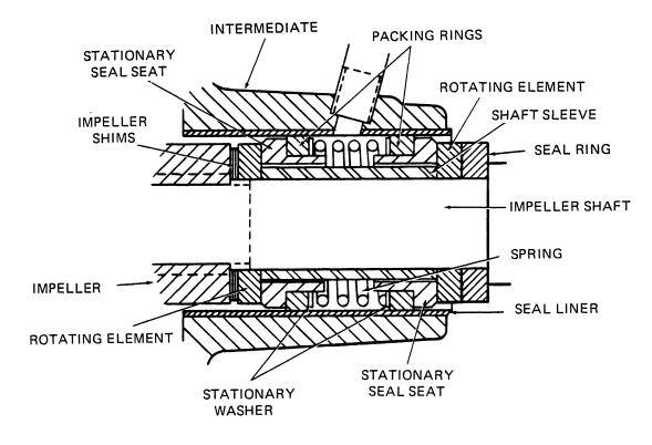
Figure 2. GS-1000 Seal Assembly
