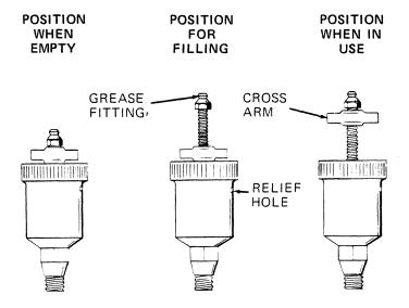
Figure 3. Automatic Lubricating Grease Cup
