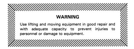
Make sure that hoists and other lifting equipment are of sufficient capacity to safely handle the pump assembly. If chains and cables are used, make certain that they are positioned so that they will not damage the pump, and so that the load will be balanced.
