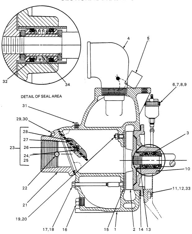
Figure 2. Pump End Assembly 83B2-ST1
