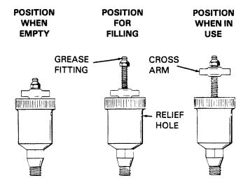
Figure 4. Automatic Lubricating Grease Cup
