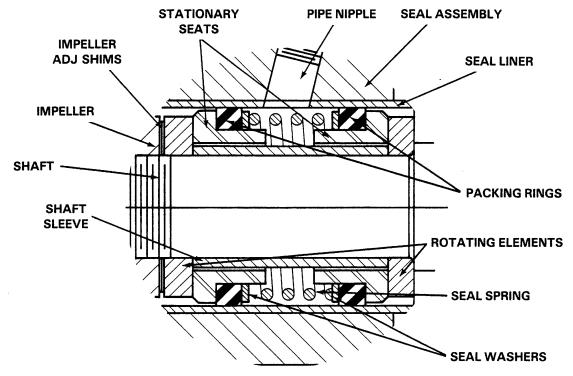
Figure 3. GS-1000 Seal Assembly
