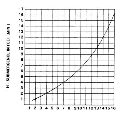
VELOCITY IN FEET PER SEC. =  $\frac{\text{QUAN. [G.P.M.] x .321}}{\text{AREA}} \text{OR} \quad \frac{\text{G.P.M. x .4085}}{\text{D}^2}$
