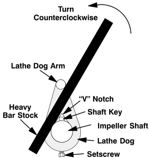
**Figure 2. Loosening Impeller**
