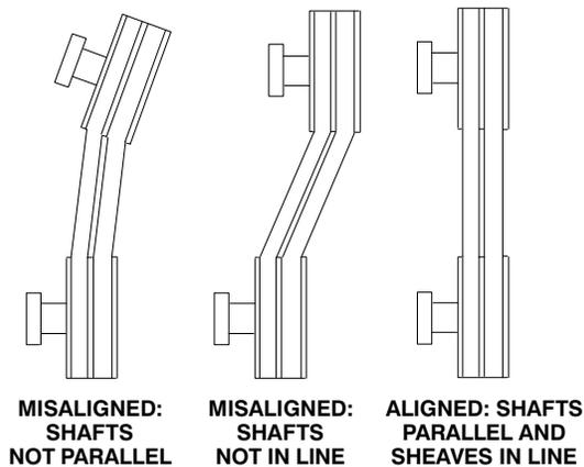
**Figure 3C. Alignment of V-Belt Driven Pumps**
