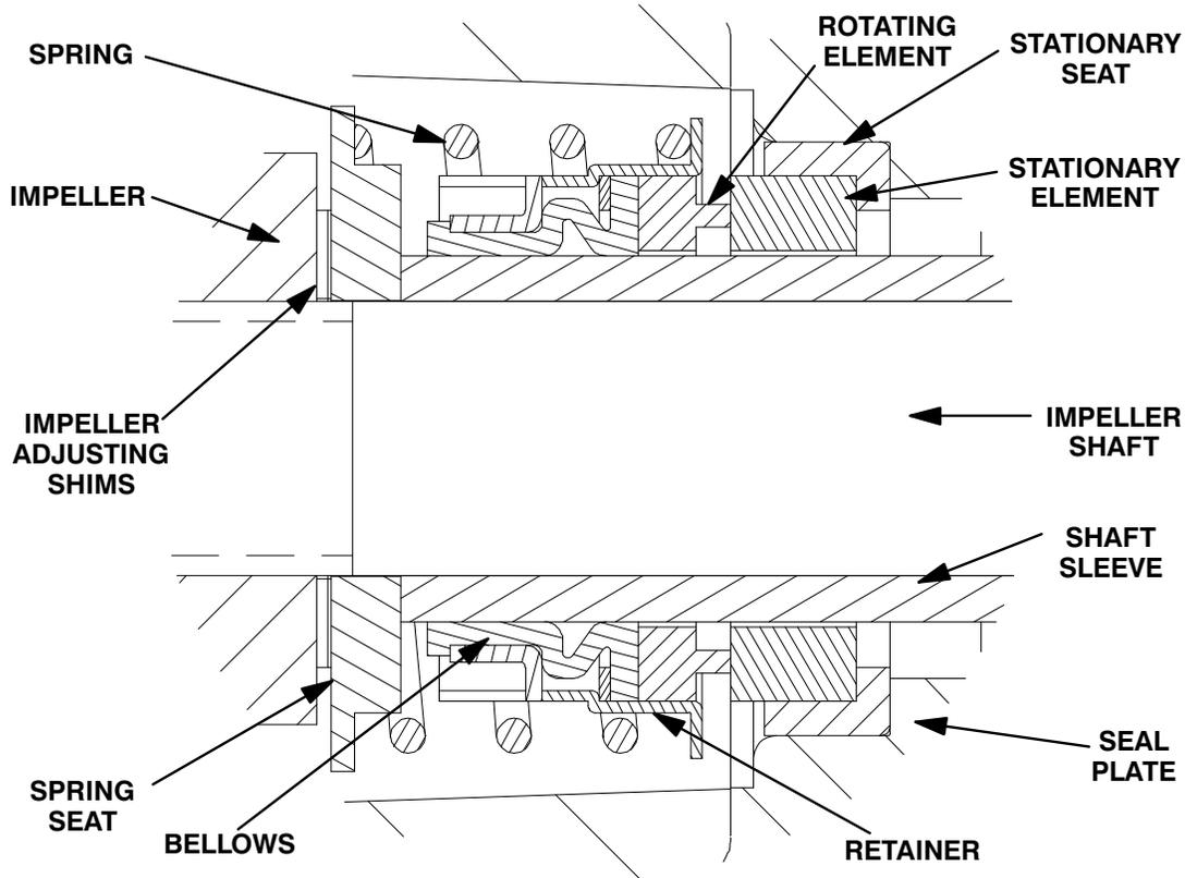
Figure 3. Seal Assembly
