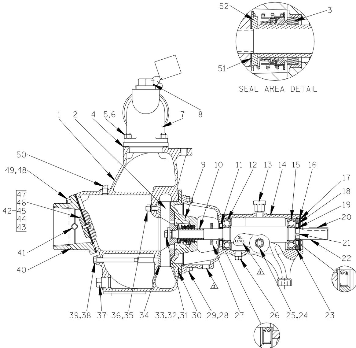
Figure 1. Pump Model 83A3-B
