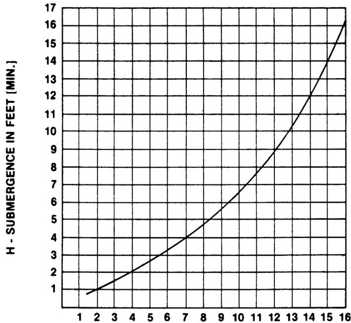
$$\text{VELOCITY IN FEET PER SEC.} = \frac{\text{QUAN. [G.P.M.] x .321}}{\text{AREA}} \text{ OR } \frac{\text{G.P.M. x .4085}}{D^2}$$
