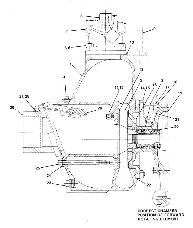
Figure 1. Pump Model 83A2-AB1
