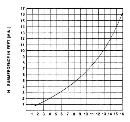
VELOCITY IN FEET PER SEC. =  $\frac{\text{QUAN. [G.P.M.] x .321}}{\text{AREA}}$  OR  $\frac{\text{G.P.M. x .4085}}{\text{D}^2}$
