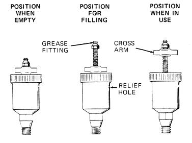
Figure 3. Automatic Lubricating Grease Cup
