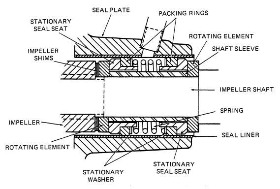
Figure 2. GS-1000 Seal Assembly
