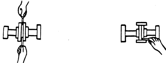
Figure 4b. Aligning Non-Spider Type Couplings
