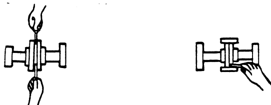
Figure 4b. Aligning Non-Spider Type Couplings
