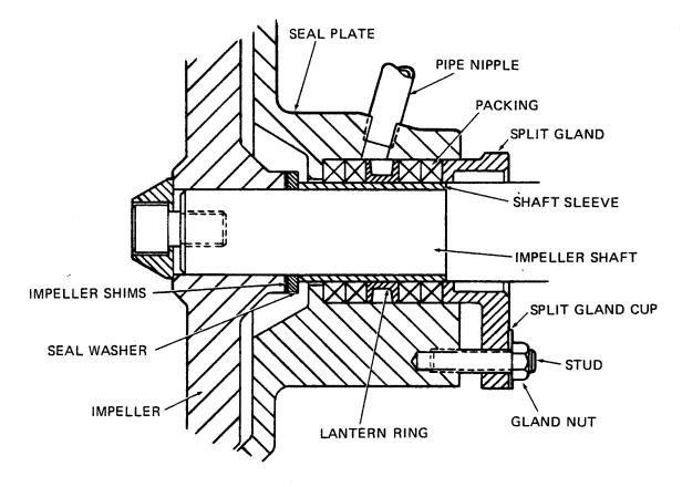
Figure 2. PP-06271/2 Packing Assembly
