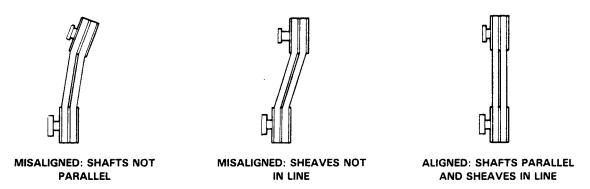
Figure 5C. Alignment of V-Belt Driven Pumps
