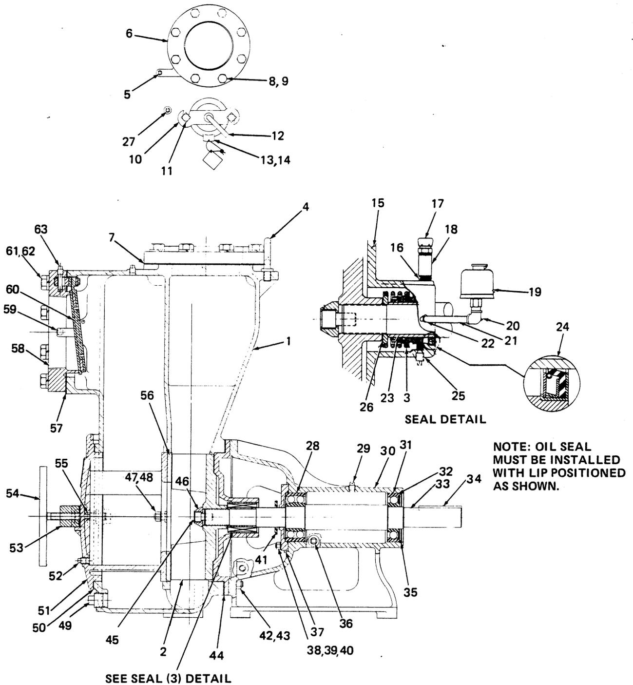
Figure 1. Pump Model 16C20-B
