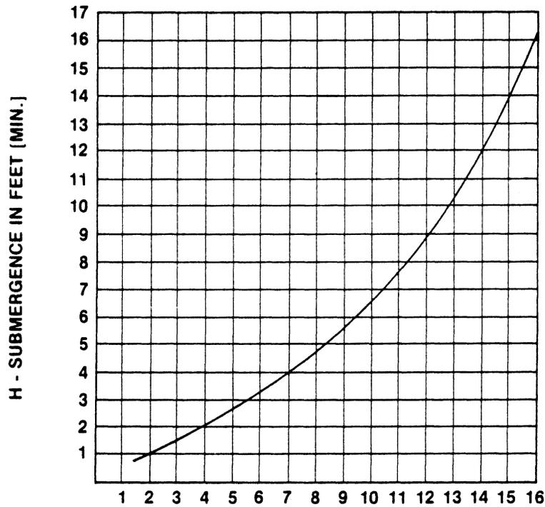
$$\text{VELOCITY IN FEET PER SEC.} = \frac{\text{QUAN. [G.P.M.]} \times .321}{\text{AREA}} \quad \text{OR} \quad \frac{\text{G.P.M.} \times .4085}{D^2}$$
