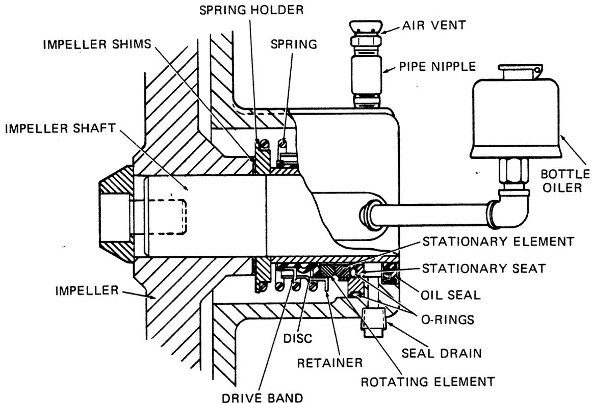
Figure 2. 12461 Seal Assembly
