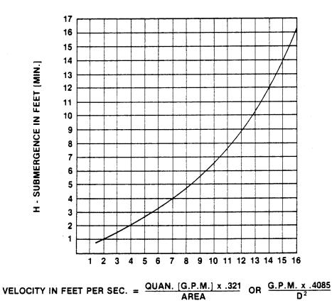
Figure 1. Recommended Minimum Suction Line Submergence Vs. Velocity
