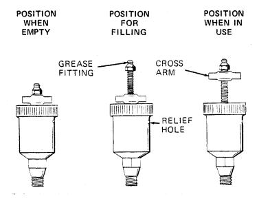
Figure 4. Automatic Lubricating Grease Cup
