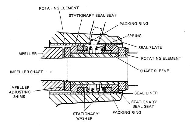
Figure 3. GS-1500 Seal Assembly
