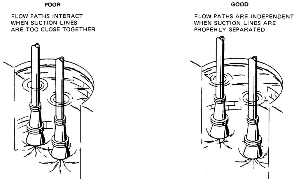
Figure 3. Using Two Pumps in the Same Sump
