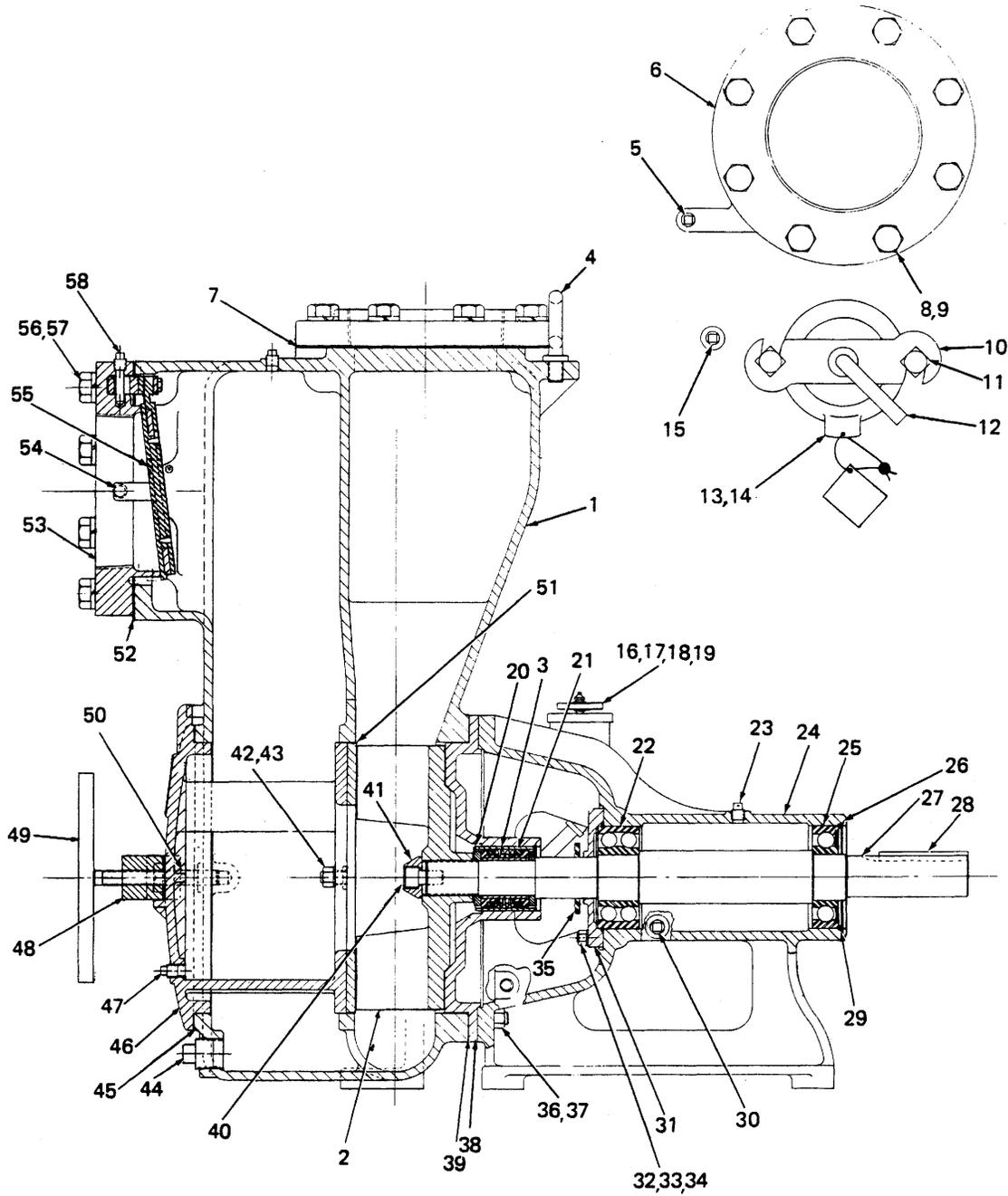
Figure 1. Pump Model 16C2-B
