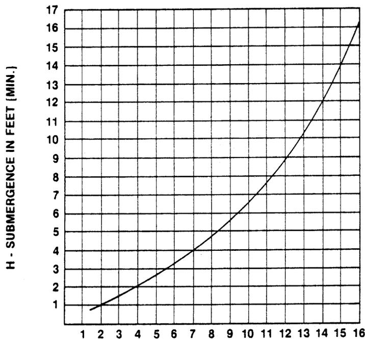
$$\text{VELOCITY IN FEET PER SEC.} = \frac{\text{QUAN. [G.P.M.] x .321}}{\text{AREA}} \quad \text{OR} \quad \frac{\text{G.P.M. x .4085}}{D^2}$$
