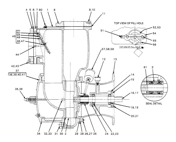
Figure 1. Model 16A2-5034 Pump End Assembly
