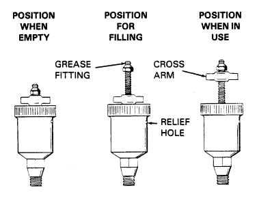
Figure 4. Automatic Lubricating Grease Cup
