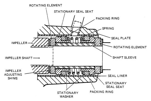
Figure 3. GS-1500 Seal Assembly
