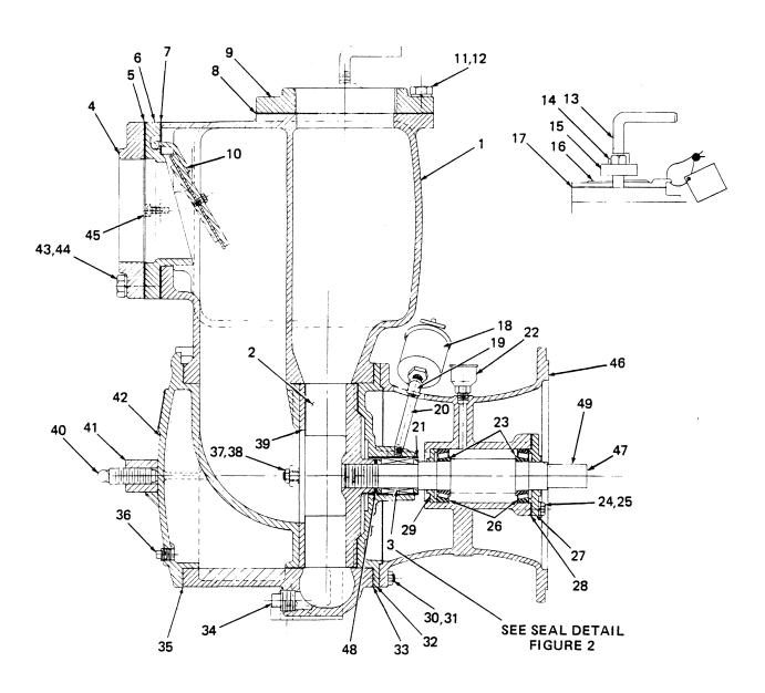
Figure 1. Pump Model 16A2-5034
