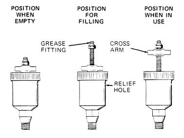
Figure 3. Automatic Lubricating Grease Cup
