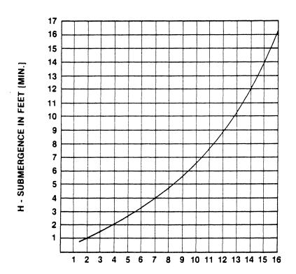
VELOCITY IN FEET PER SEC. =  $\frac{\text{QUAN. [G.P.M.] x .321}}{\text{AREA}} \text{ OR } \frac{\text{G.P.M. x .4085}}{\text{D}^2}$
