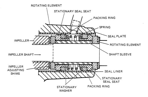
Figure 2. GS-1500 Seal Assembly
