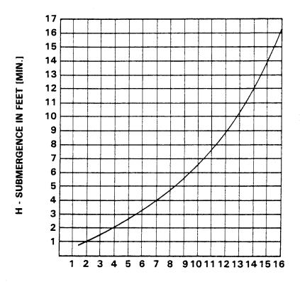
VELOCITY IN FEET PER SEC. =  $\frac{\text{QUAN. [G.P.M.]} \times .321}{\text{AREA}}$  OR  $\frac{\text{G.P.M. x} .4085}{\text{D}^2}$
