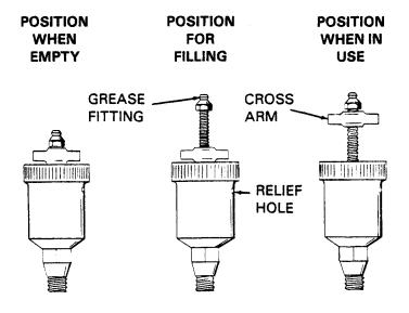
Figure 3. Automatic Lubricating Grease Cup
