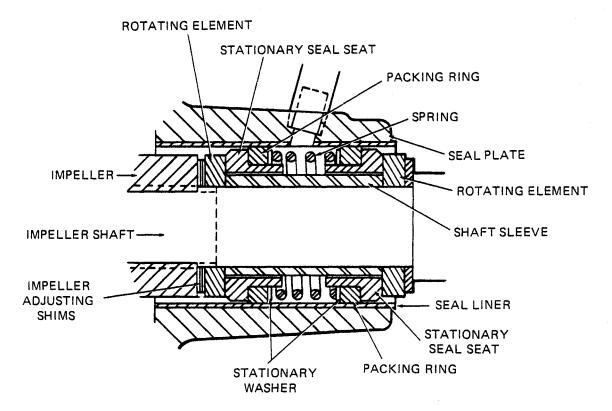
Figure 2. GS-1500 Seal Assembly
