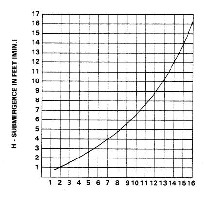
VELOCITY IN FEET PER SEC. =  $\frac{\text{QUAN. [G.P.M.] x .321}}{\text{AREA}} \text{OR } \frac{\text{G.P.M. x .4085}}{\text{D}^2}$
