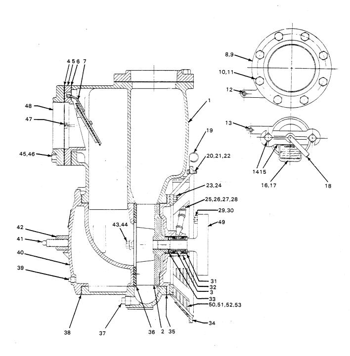
Figure 1. Pump End Only Model 16A2-HR3
