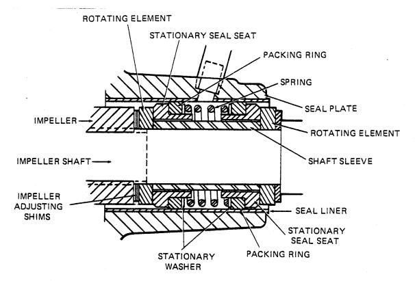
Figure 2. GS-1500 Seal Assembly
