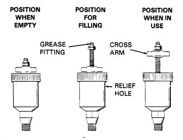
Figure 3. Automatic Lubricating Grease Cup
