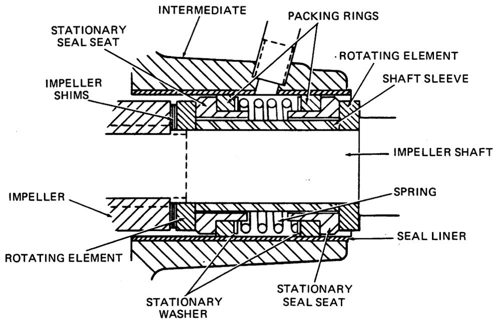
Figure 4. GS-1500 Seal Assembly
