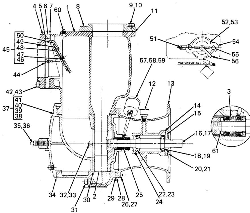
Figure 3. Pump End Only Model 16A2
