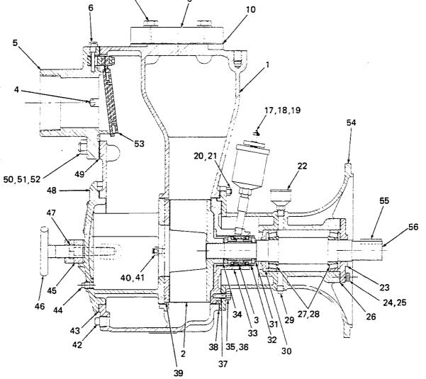
Figure 1. Pump Model 14C2-DD
