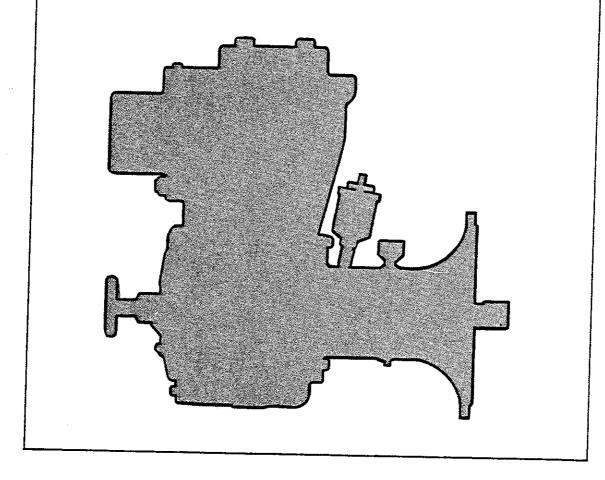
The only moving parts of this pump are the impeller, seal rotating elements, and the shaft. The wear plate, impeller, and seal, which receive the most wear, are easily accessible and can be replaced without disturbing the piping. Maintenance and replacement of these three parts will maintain the peak operating efficiency of the pump.
