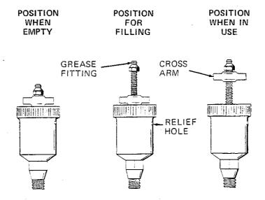
Figure 3. Automatic Lubricating Grease Cup
