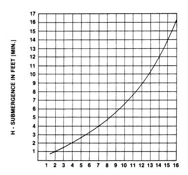
VELOCITY IN FEET PER SEC. =  $\frac{\text{QUAN. [G.P.M.]} \times .321}{\text{AREA}} \quad \text{OR} \quad \frac{\text{G.P.M.} \times .4085}{\text{D}^2}$
