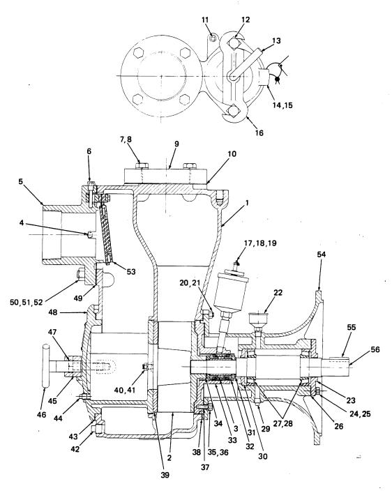
Figure 1. Pump Model 14C2-D
