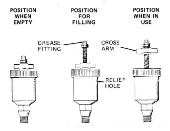
Figure 3. Automatic Lubricating Grease Cup
