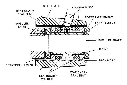
Figure 2. GS-1250 Seal Assembly
