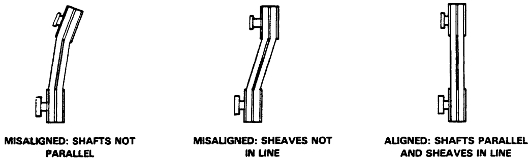
Figure 3C. Alignment of V-Belt Driven Pumps
