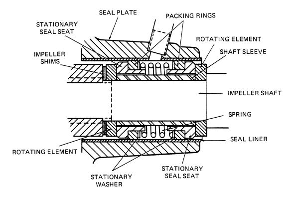
Figure 2. GS-1250 Seal Assembly
