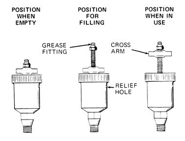
Figure 3. Automatic Lubricating Grease Cup
