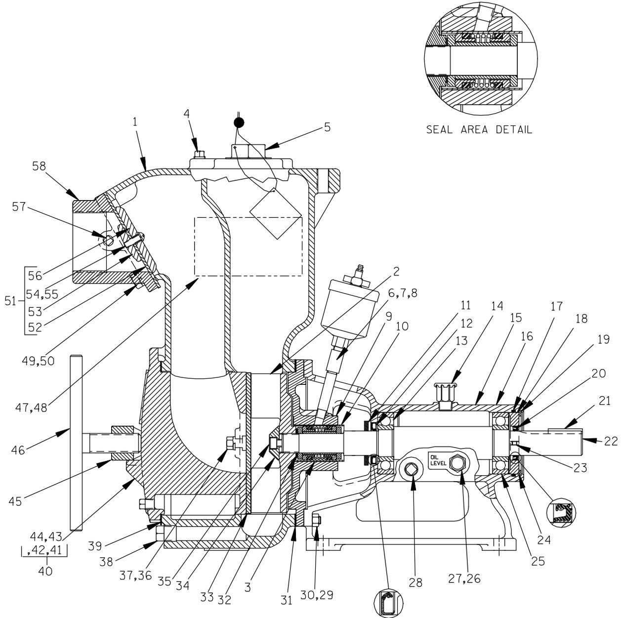
Figure E-1. Pump Model 13A2-B
