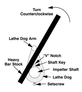
Figure 2. Loosening Impeller
