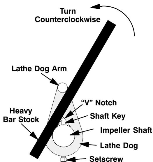
**Figure 2. Loosening Impeller**
