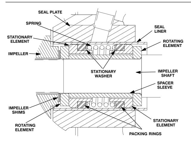
Figure 3. Seal Assembly
