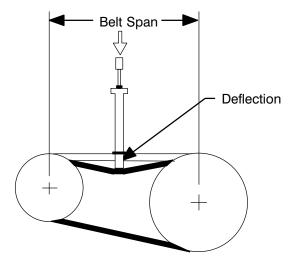
Figure 5. Belt Tension Measurement
