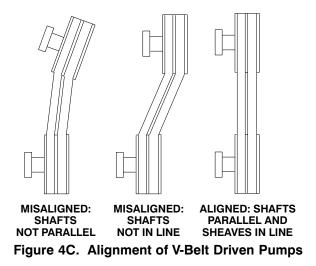
Tighten the belts in accordance with the belt manufacturer's instructions. If the belts are too loose, they will slip; if the belts are too tight, there will be excessive power loss and possible bearing failure. Select pulleys that will match the proper speed ratio; overspeeding the pump may damage both pump and power source.
