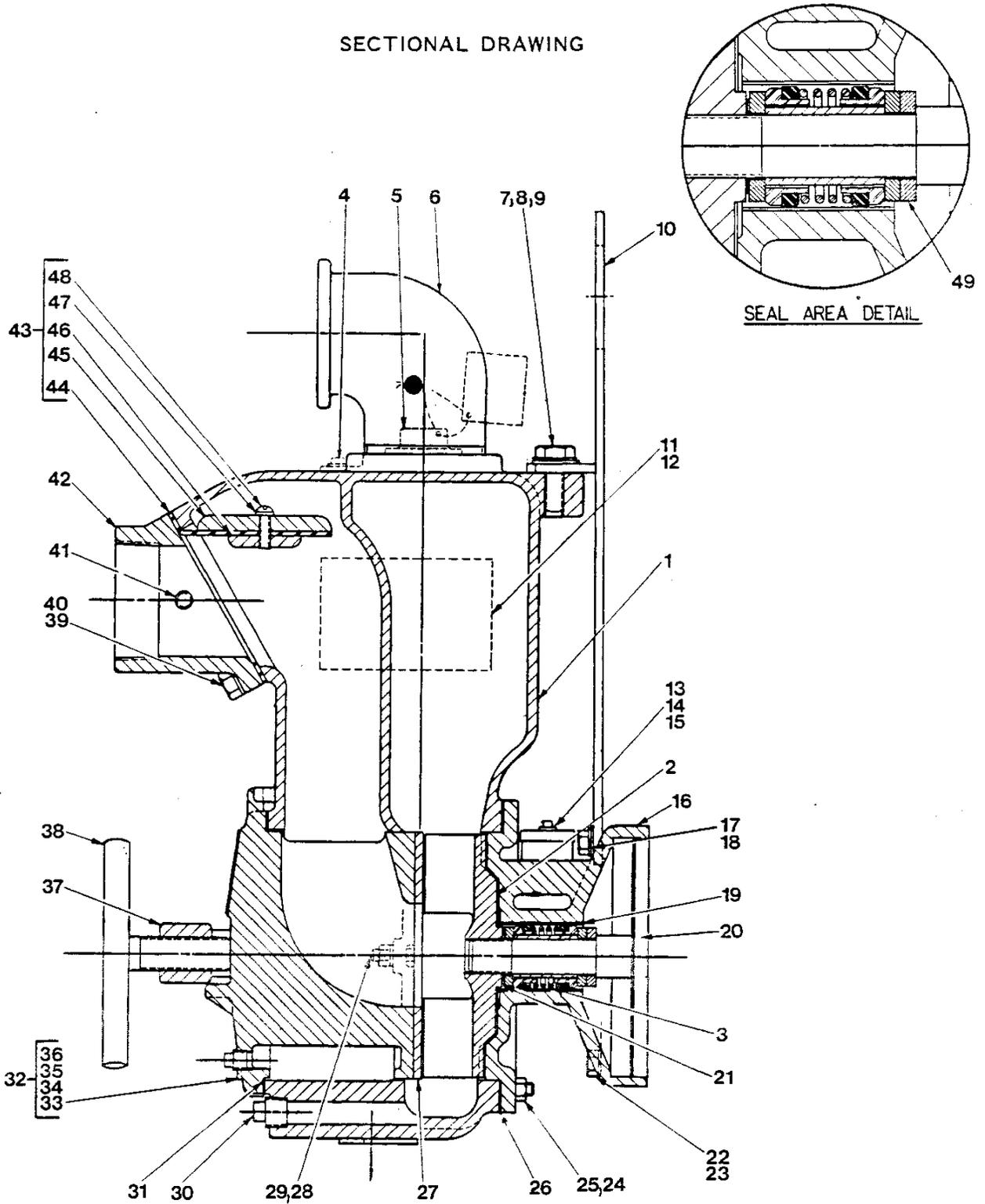
Figure 2. Pump End Assembly 13A2-(AENLD S/G)
