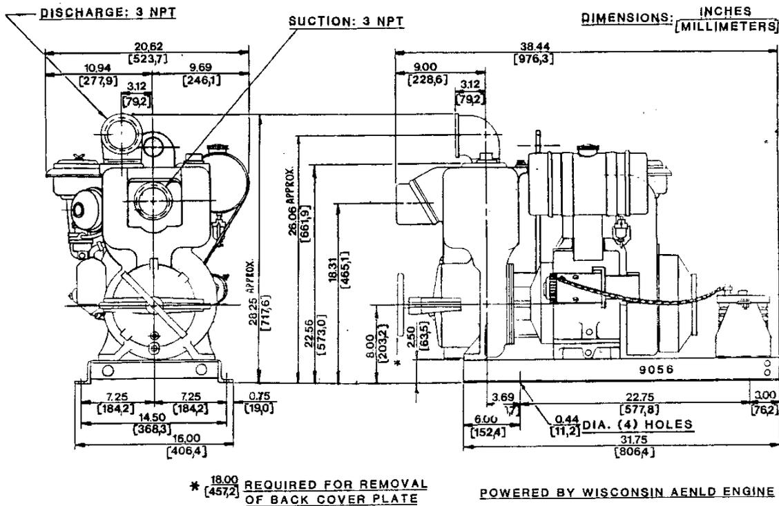
Figure 1. Pump Model 13A2-AENLD S/G
