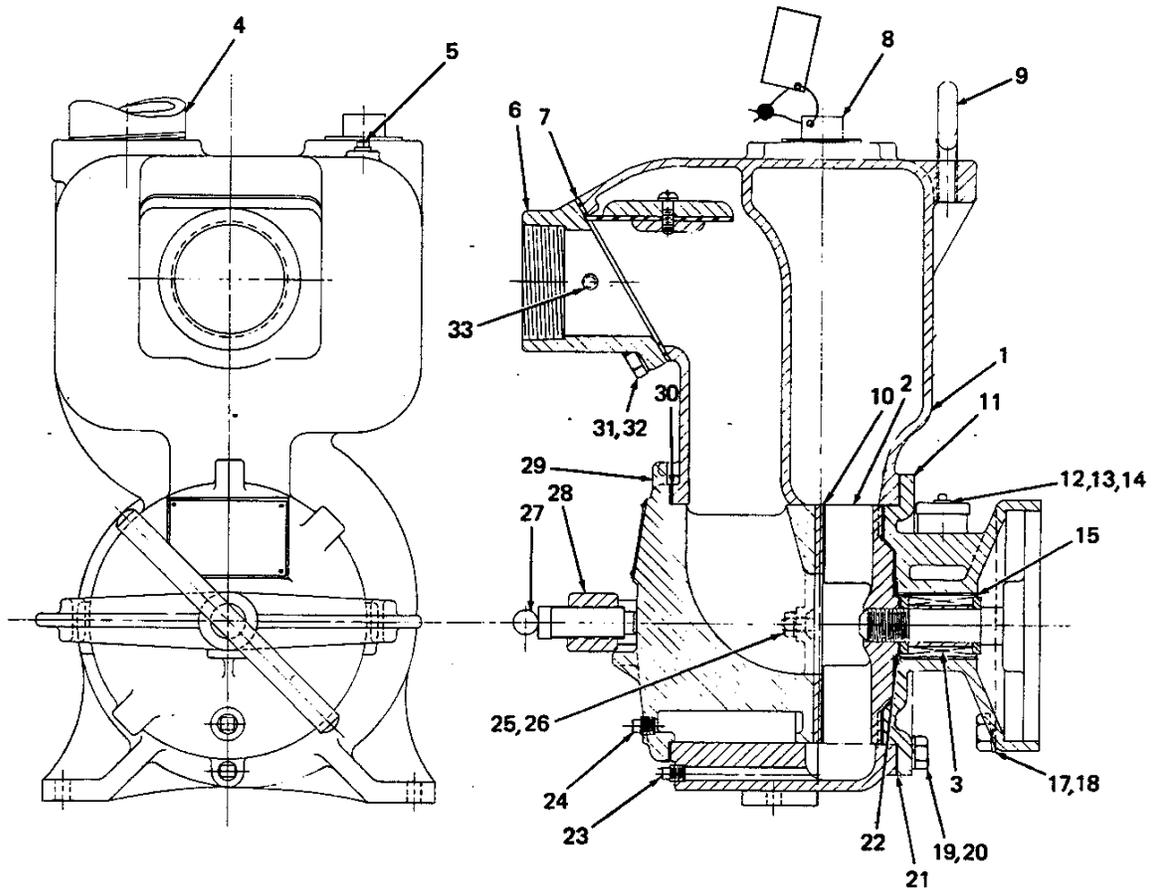
Figure 1. Pump Model 13A2-AENLD S/G
