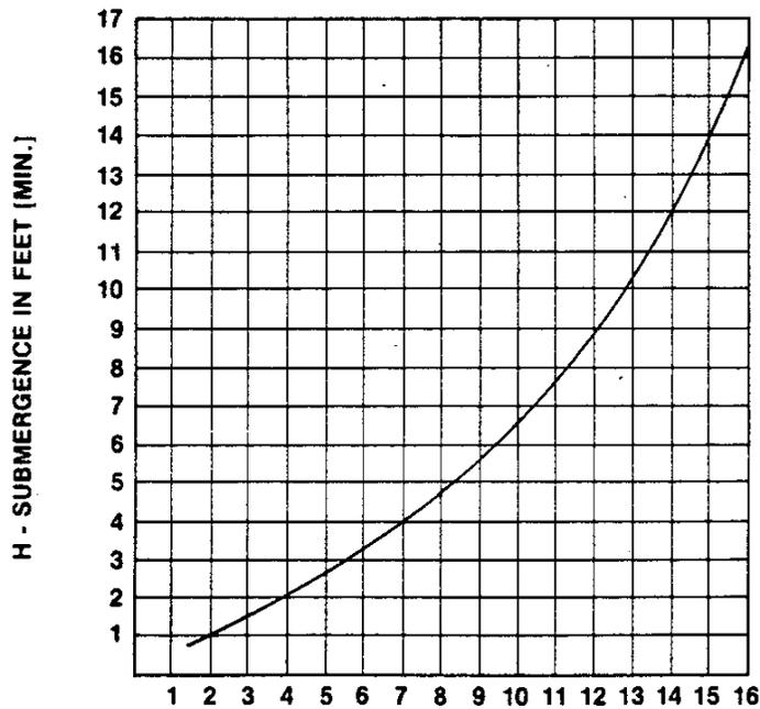
$$\text{VELOCITY IN FEET PER SEC.} = \frac{\text{QUAN. [G.P.M.]} \times .321}{\text{AREA}} \text{ OR } \frac{\text{G.P.M.} \times .4085}{D^2}$$
