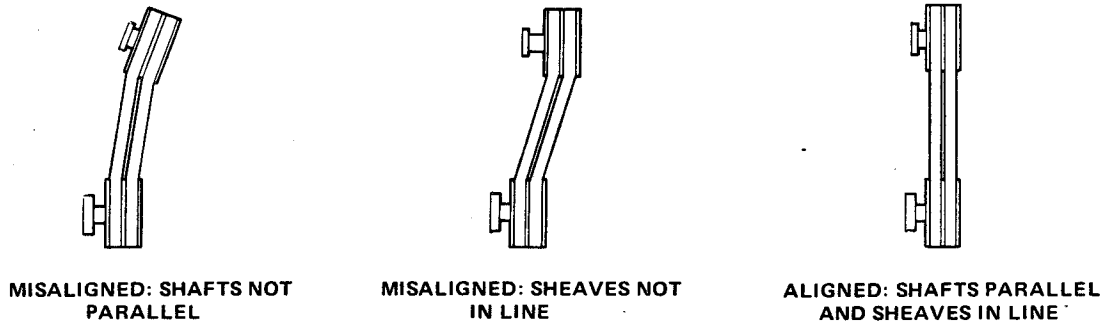
Figure 5C. Alignment of V-Belt Driven Pumps
