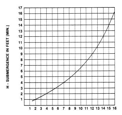
VELOCITY IN FEET PER SEC. =  $\frac{\text{QUAN. [G.P.M.]} \times .321}{\text{AREA}}$  OR  $\frac{\text{G.P.M.} \times .4085}{\text{D}^2}$
