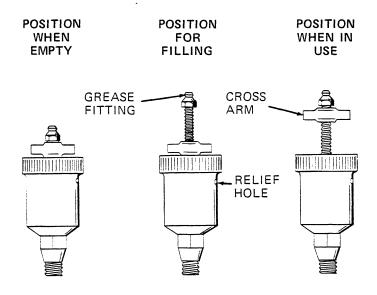
Figure 3. Automatic Lubricating Grease Cup
