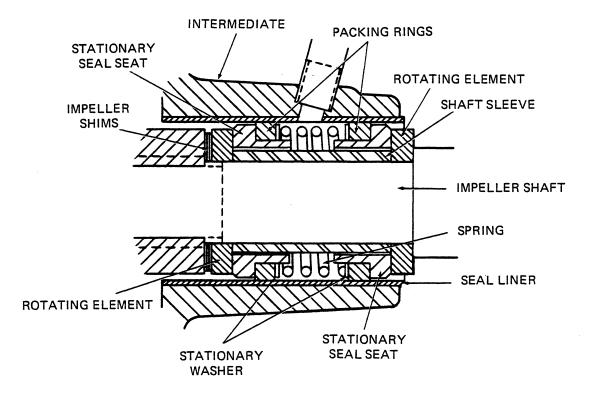
Figure 2. GS-1000 Seal Assembly
