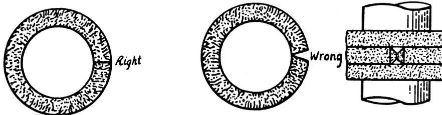
**Step 2:** It is critical that the ends of the cut packing rings meet in a tight parallel fit to ensure proper sealing. Check this fit; it should be correct if the packing was cut while wrapped around a rod, but if the packing was cut while laid out straight, the ends will meet at an angle. **Never** install a packing ring with an angled gap; pressure on adjacent packing rings will cause them to work into the gap and prevent the angled ring from closing properly around the shaft.
