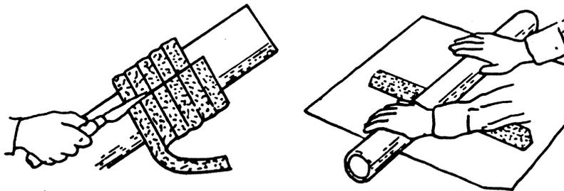
**Step 1:** Determine how much bulk packing will be required to fill the packing cavity, and wrap it around a rod of the same diameter as the shaft. With the packing wrapped around the rod, cut through each turn as shown.
