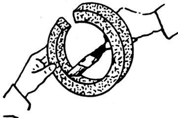
**Step 3:** Lubricate all metallic packings (foil type, lead core, etc.) with the lubricant recommended by the packing manufacturer. Generally, swabbing the inside diameter of this type packing with SAE No. 30 non-detergent oil provides sufficient lubrication.
