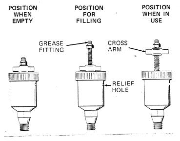
Figure 3. Automatic Lubricating Grease Cup
