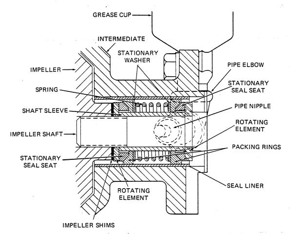
Figure 2. GS-625 Seal Assembly
